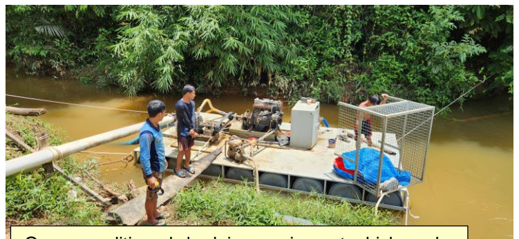
Our reconditioned dredging equipment which sucks up all the river sand for our concrete plant.
